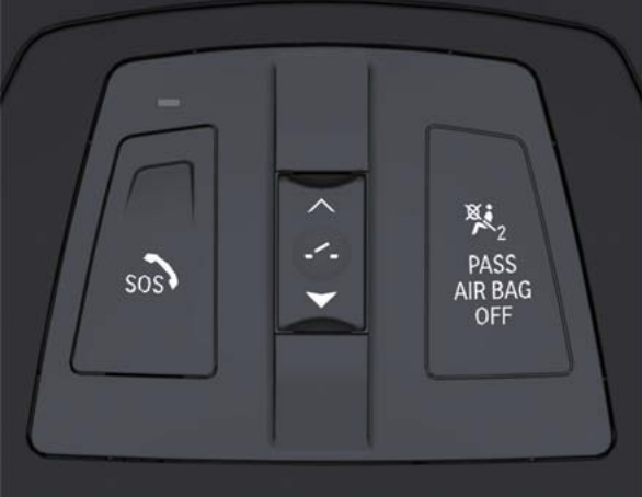
F10 Roof function center with indicator lamp for front passenger airbag deactivation
